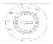
Fig4 (Rotary Time Control Switch)
